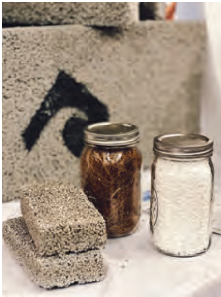
Waste material from surfboards is deconstructed and poured into molds for building blocks.
