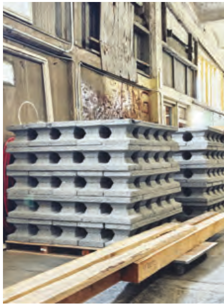
Waste material from surfboards is deconstructed and poured into molds for building blocks.
