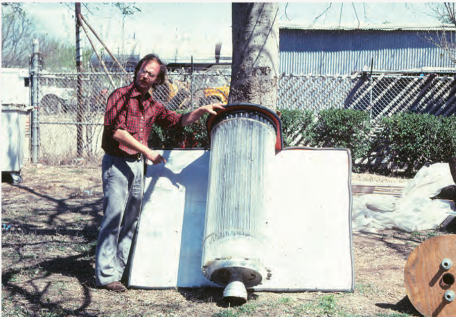
Fisk can be seen here with a finished solar heater for residents of Crystal City. The old tanks were wrapped in plastic and fluorescent light tubes, set above reflective plates to generate heat when installed on the roof as a complete unit.
