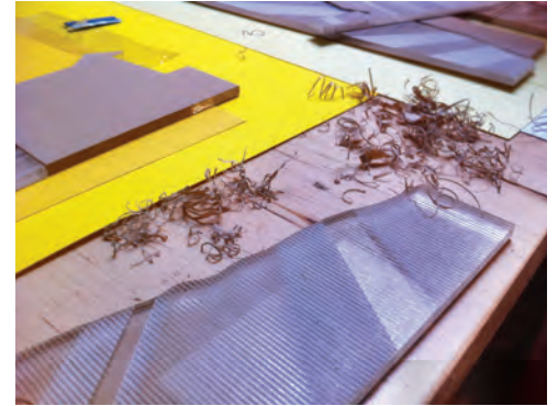
Below The right depth of engraving is critical to ensure a deep impression without warping the acrylic plates used to make the prints. A misalignment of as little as a 32nd of an inch in the line work could result in a shifted color pattern and an undesirable result.
