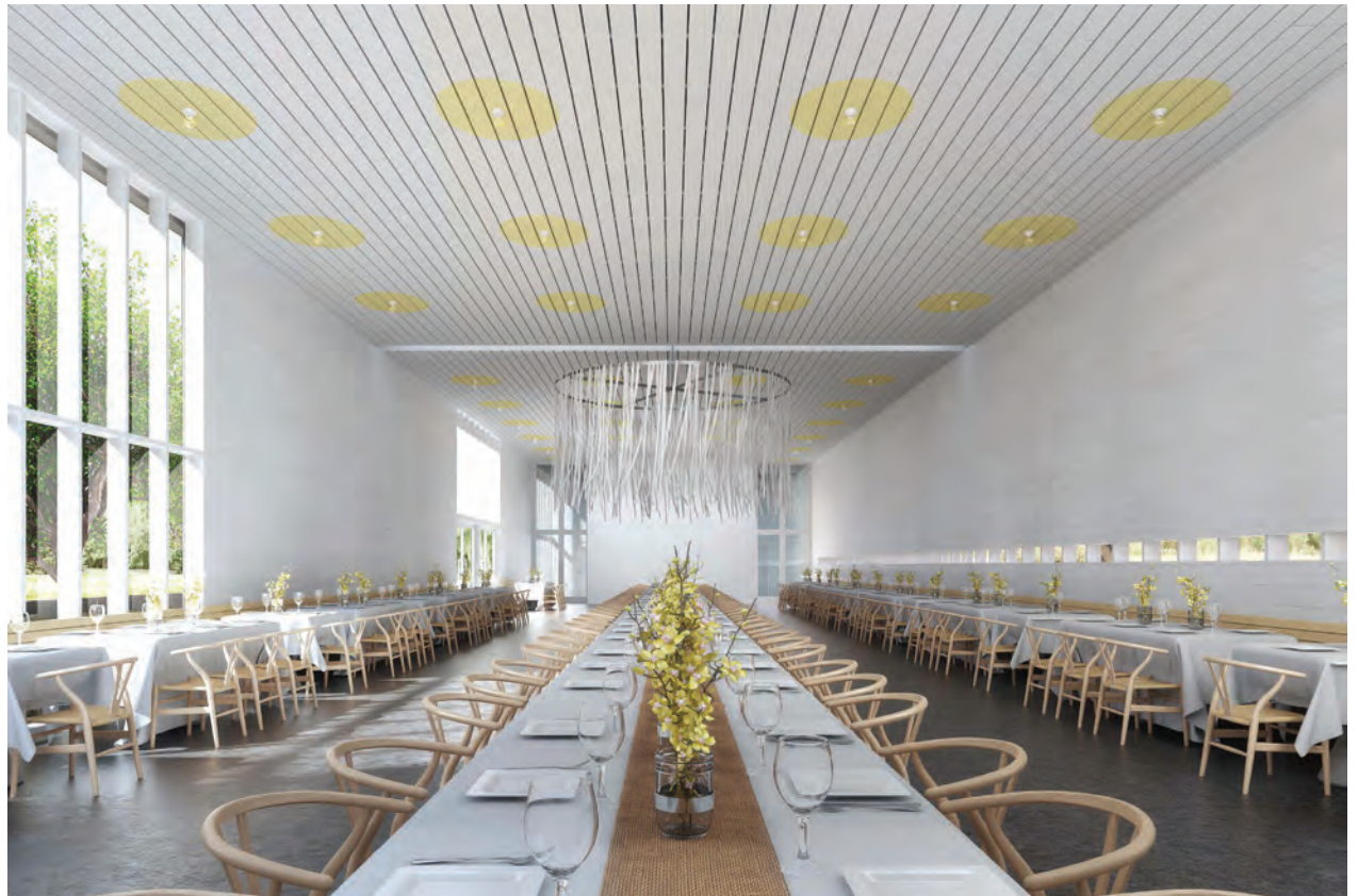
Rendered view of the main hall with the wind vane chandelier attached to the wind vane on the roof.
