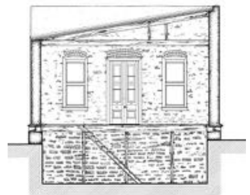
UTSA students took measurements of the Heermann Store prior to producing a set drawings based on the standards of the Historic American Building Survey. The one-room structure of load-bearing, rough-cut, coursed blocks of red sandstone dates from 1892 and was erected along the Rockport Road (now re-aligned to form Loop 1604 in southwest Bexar County), which connected Castroville and the Texas coast.
