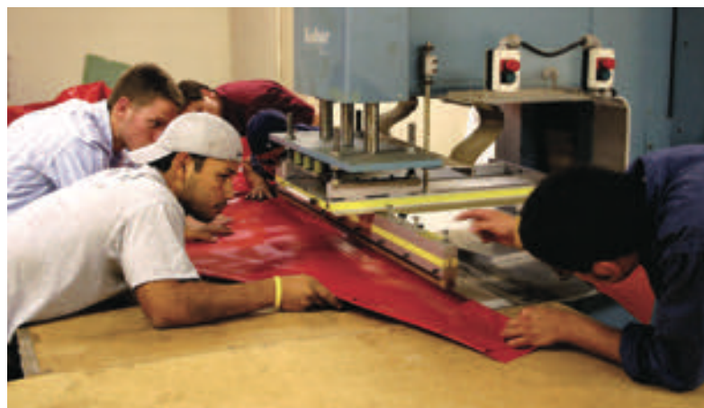
A second permanent installation of tensile membrane structure serves as an entrance canopy. Specialized software was used to design and fabricate the components that students cut and stitched at workshops whose owners helped sponsor the project.
