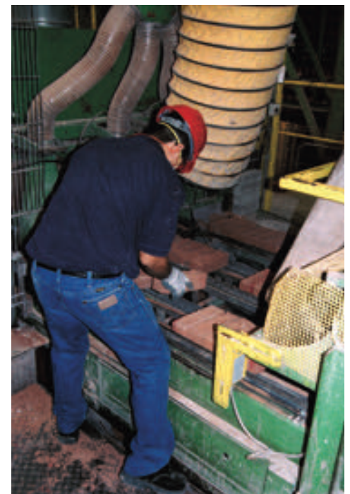
(above) Three varieties of machine-molded bricks from Acme's Elgin plant are shown in front of a wall built of handmolded, gas-fired brick from Reynosa Brick Company. (below) A worker at the Elgin plant intervenes in the dryer-car unloading process to double and group unloaded dried bricks into layers prior to being transported by robotic equipment into a kiln. Earlier this year Acme switched to a different technology at the Elgin plant.
