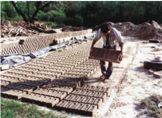
Brickmaking at Ladrillera La Paloma in Reynosa begins by mixing the local clay and placing it into molds. The unfired bricks are then emptied from the molds onto dirt surfaces for drying before they are loaded into a kiln.
