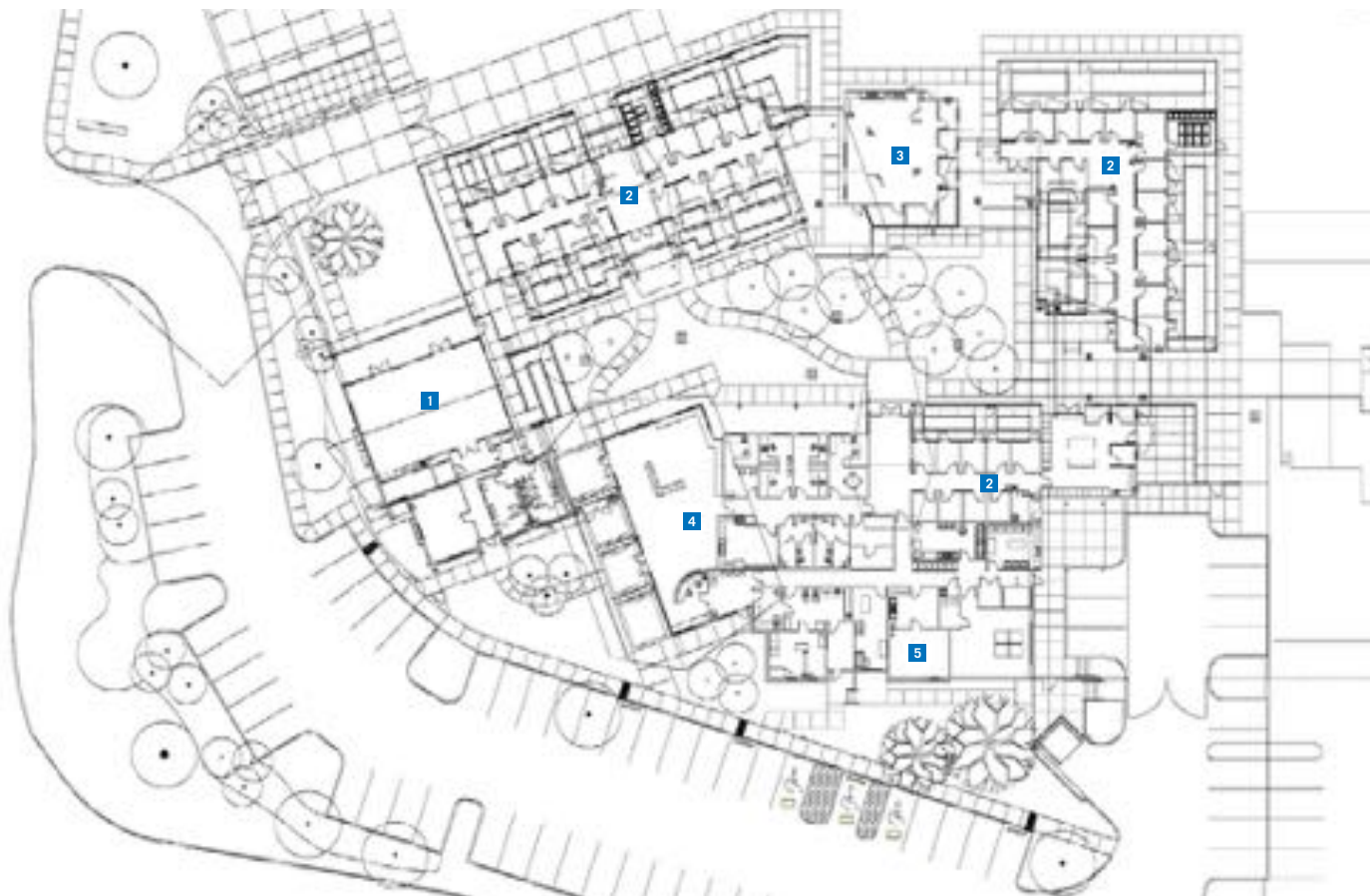
SITE PLAN 1 EDUCATION BUILDING 2 CANINE ADOPTION 3 FELINE ADOPTION 4 ADOPTION LOBBY AND ADMINISTRATION 5 RECEIVING LOBBY, CLINIC, AND BACK OF HOUSE
