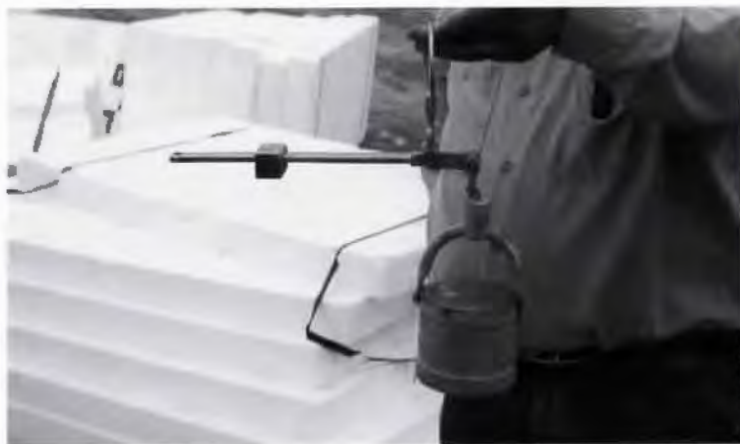
Testing wet density
