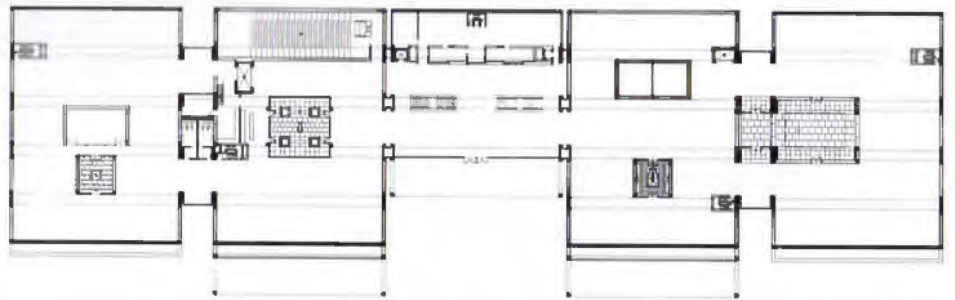
Giurgola's schematic design adds two new five-vault wings (view from southwest, ABOVE; plan, BELOW).
