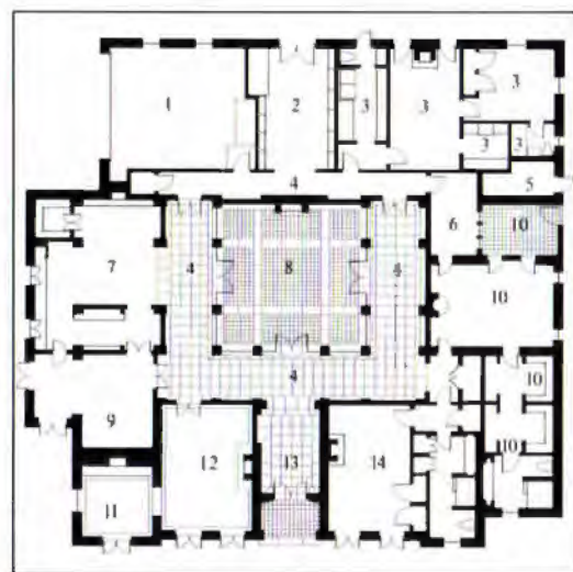
Lifshutz residence, floor plan: 1: garage; 2: workroom; 3: servant's suite; 4: galleries; 5: mechanical; 6: studio; 7: kitchen; 8: courtyard; 9: dining; 10: master suite; 11: secrets room; 12: living room; 13: entry; 14: guest bedroom
