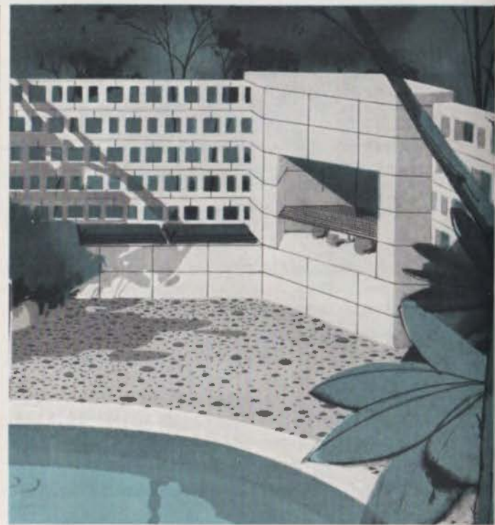
SCREEN WALL OF CONCRETE MASONRY. Lacy pattern is created from sections of standard block. Planters to patios, concrete can be both high-style and practical.
