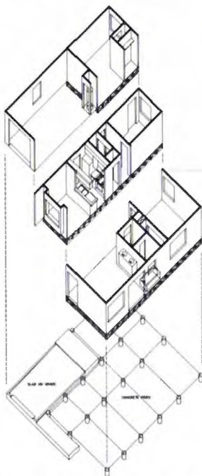
The homes are built in sections at a plant, then brought to the site and assembled on piers that are poured in place.
