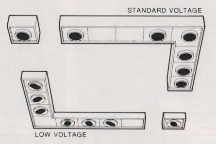
Modular Adjustable Systems are available in standard and low voltage types, surface mount or recessed. 1 by 1 foot fixtures and blank plates can be relocated at will, quickly and without tools, to keep pace with changing displays and exhibitions.
