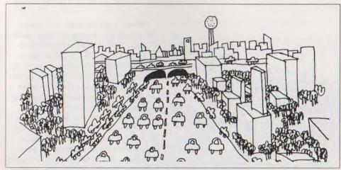
freeway with a second freeway (primarily for buses), and constructing a fixed rail transit line elevated above the center median.
