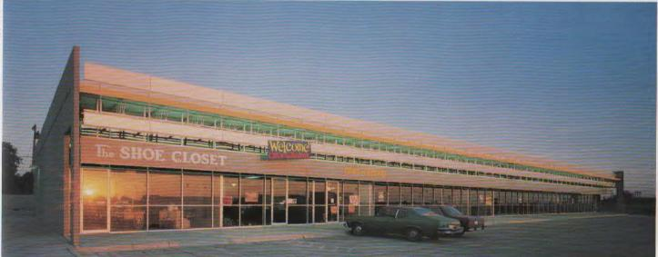
Retail Strip, Beltline at Grande, Parkey & Partners. Stripped down strip with a dressy canopy, parasitic to Irving Mall. Innovative use of steel bar joist construction. Front glass wall is set back to create protective overhang. Four parallel bands—mechanical screen above, yellow trim cap, light valance, and grey sign band—complete and decorate the canopy while accentuating horizontality. Above eight feet, mirror glass augments the intricacy of exposed structure and the play of light within it.
