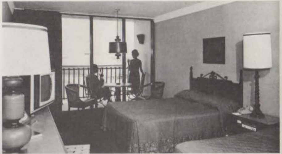
Typical completed unit with all furnishings and finishes installed before delivery to jobsite.
