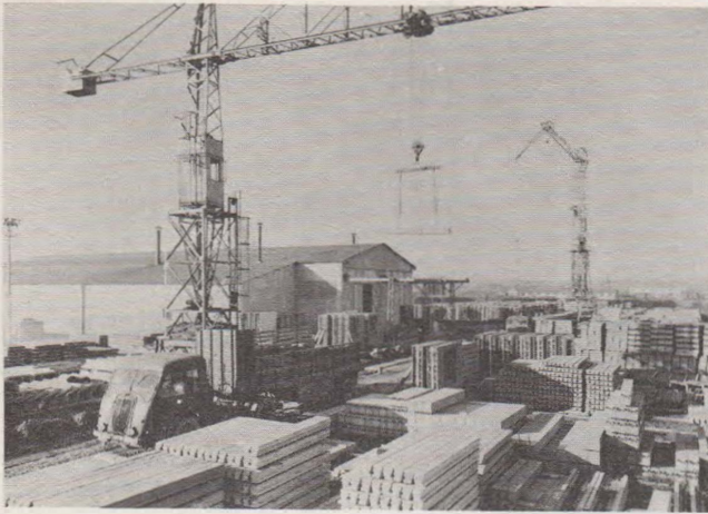
In Europe prefabricated prestressed clay masonry structural elements are plant made and inventoried.
