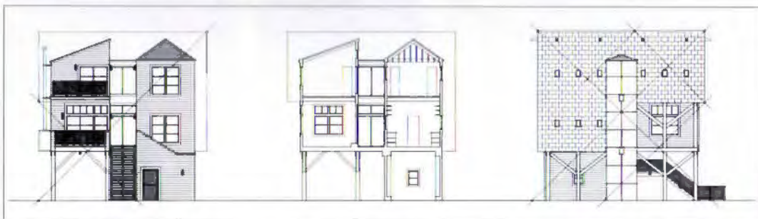
Highway House, ABOVE: (left to right) elevation, section, elevation; BELOW: plans, with first floor at left, roof at right
