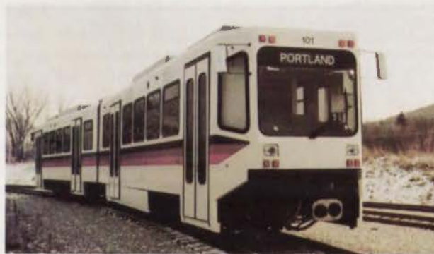
The Portland system will employ this articulated light rail vehicle produced by Bombardier Inc., Quebec. Less capital-intensive than heavy rail, light rail transit is the likely choice for applications in Texas.
