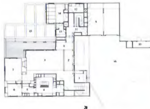
First floor: 1. entry/porch, 2. gallery, 3. living room, 4. kitchen, 5. pantry, 6. breakfast room, 7. dining room, 8. bar, 9. garage, 10. garden shed, 11. rear entry, 12. utility, 13. vanity/bath, 14. music room, 15. terrace, 16. car court.
