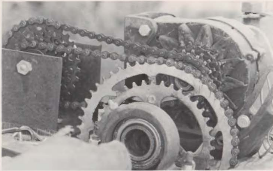
Old bicycle parts being recycled as components in a wind-powered electrical generator. Below: an early prototype is raised at the lab.
