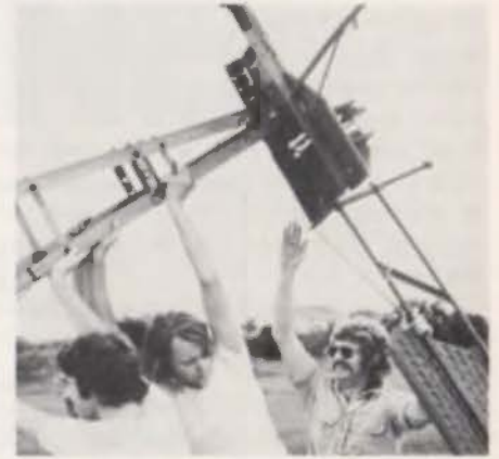
Old bicycle parts being recycled as components in a wind-powered electrical generator. Below: an early prototype is raised at the lab.
