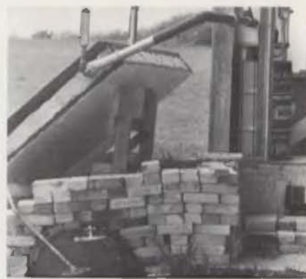
A methane digester (bio-gas plant) in service at the lab. Solar collector heats organic waste material in drum below, producing gas which is piped to the kitchen stove.
