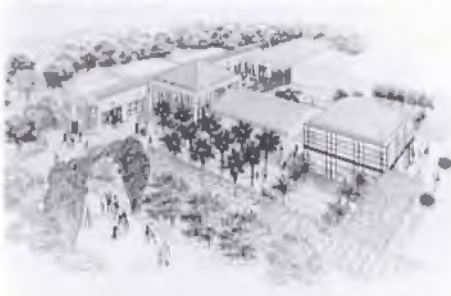
A connective spine serves as a datum for the center's activity rooms and support spaces. A geometrically abstracted serpentine water feature was retained, although two structures for a fish habitat were removed from the final design (compare plan, LEFT, with axonometric, ABOVE).
