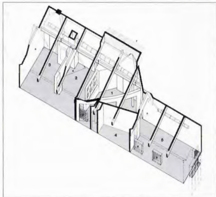
ABOVE: Axonometric shows office areas: 1-reception, 2-business office, 3-conference, 4-darkroom, 5-production studio, 6-new clerestory, 7-roof monitor, 8-new window, 9-business hallway. BELOW: plan
