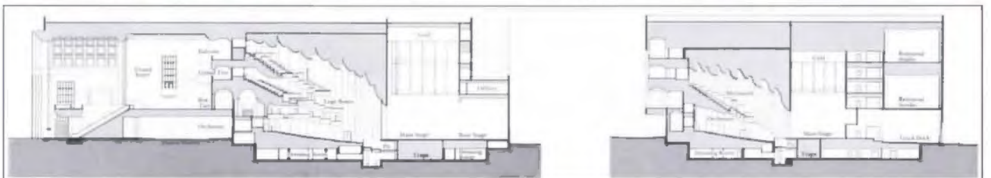
Sections, (left) through the Grand Foyer and Alice and George Brown Theater, and (right) through the Lillie and Roy Cullen theater.
