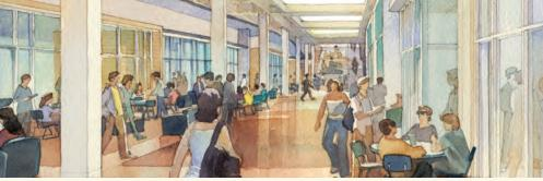
flanking flexible spaces and classrooms, the central corridor guides both people and light into the building. The floor plate above the hallway will be removed in rectangular sections, creating a linear lightwell illuminated by a new series of clerestory windows to be installed in the roof above.
