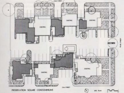
Plan: building in two phases allowed construction of two continuous structures around the courtward.
