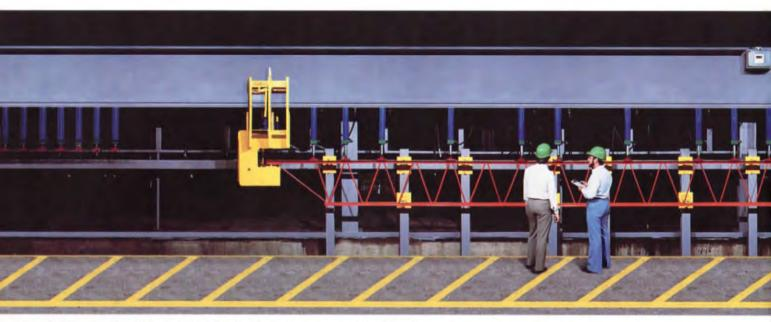
A joist is tested using the highly sophisticated, full scale load tester developed by Vulcraft.
