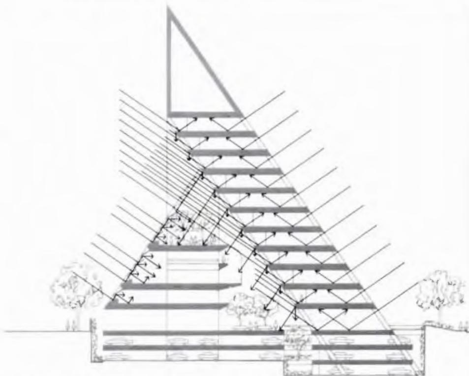
ABOVE: Building form scoops up breezes (the Malkaf Concept) and natural light. A computer would regulate air conditioning and lighting according to outside conditions. BELOW: Office space section illustrates views and ventilation.
