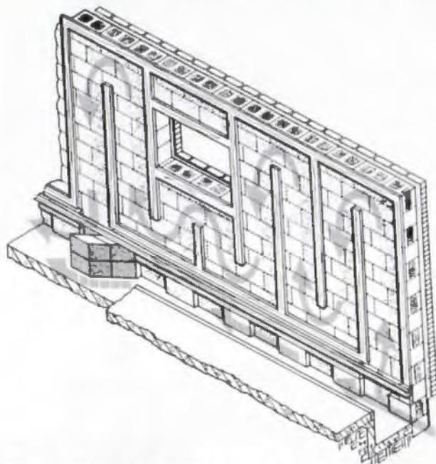
Diagram shows air pass to be covered by wallboard and flooring. Air is drawn over the wall surface through spaces created by strategic placement of furring strips. In summer, the air is mechanically cooled only at night, when low, non-peak-load utility rates are in effect. The massive walls stay cool through the day.
