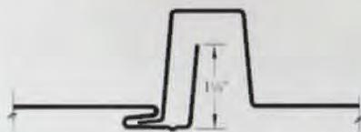
And the panels, offered in 12, 15 or 18 inch widths, are all held down with our unique concealed stainless-steel clip. A clip that per-
