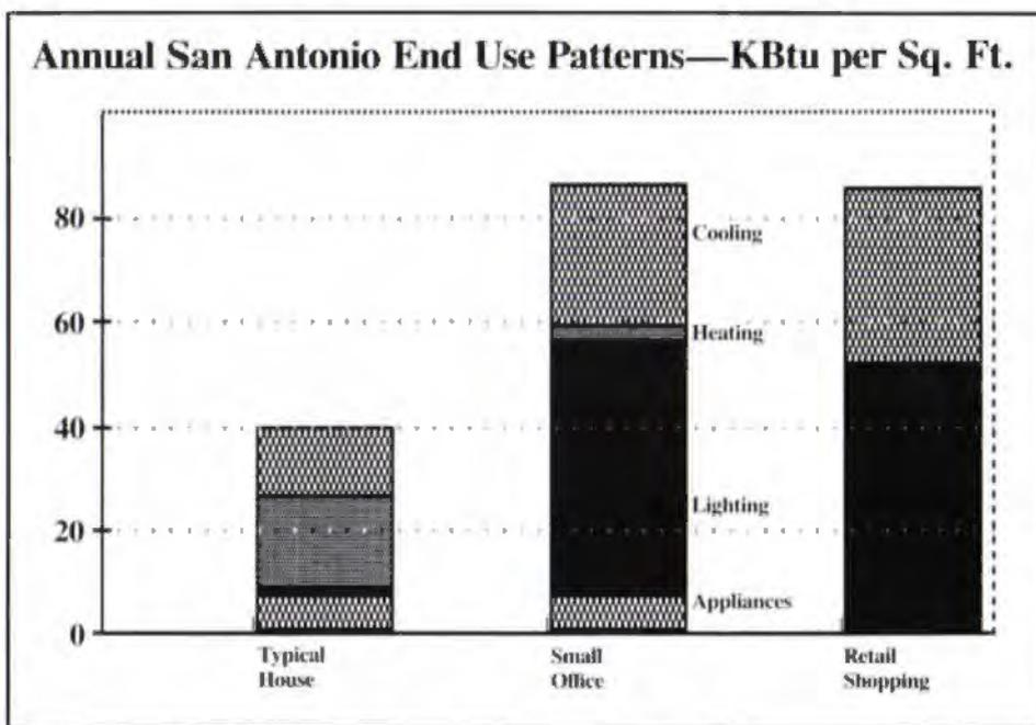
Figure 1—End-use breakouts for a San Antonio-type climate.
