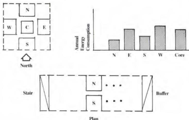
Figure 2—“Building Block” study to determine aspect ratios and orientation.
