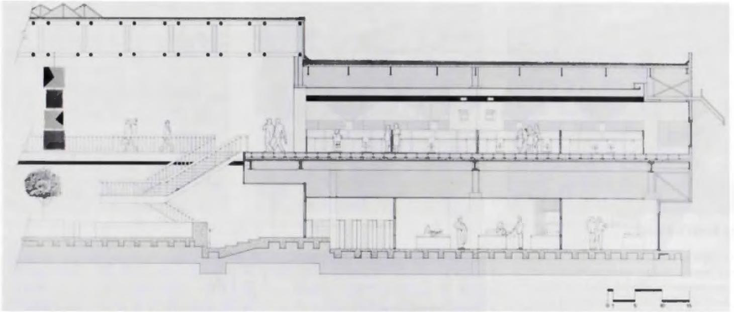
*ABOVE: Section. BELOW: "Eyebrows" extend outward six feet, reducing heat gain and minimizing glare on CRT screens.*
