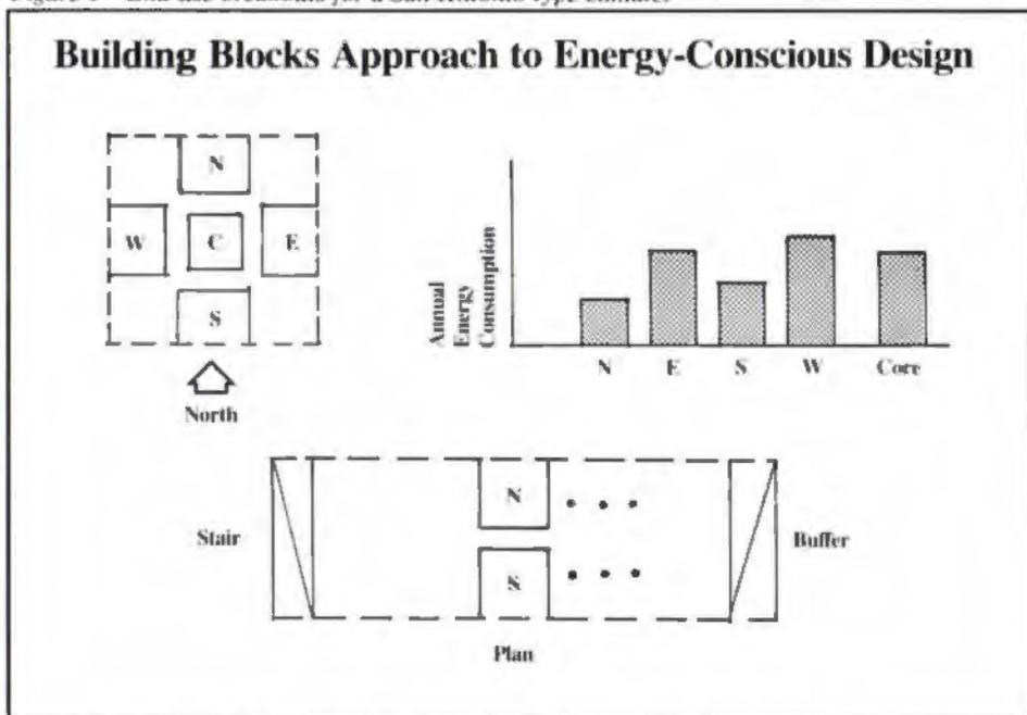
Figure 2—“Building Block” study to determine aspect ratios and orientation.
