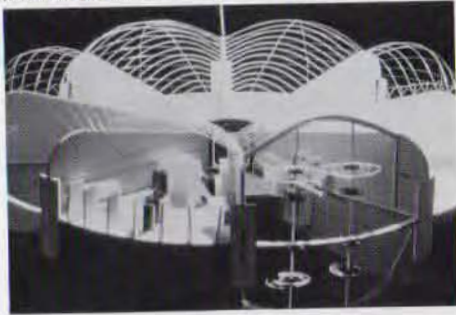
Model of inflated pod shows food preparation area at left and adjoining dining area. There are two dining levels, but no floor separating them. Astronauts would attach food trays to circular clustered mounts and anchor themselves to foot rings below.
