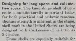
Dome shells are especially suitable for structures such as gymnasiums where spans are long and column-free space is required. As seen from the table below, shell thickness varies with length of span and curvature of dome.
