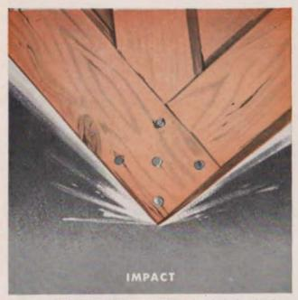
TRAFFIC AND TYPE OF EQUIPMENT dictate the floor hardness required. Typical problems include traffic wear, excessive abrasion, moisture penetration and chemical deterioration.
