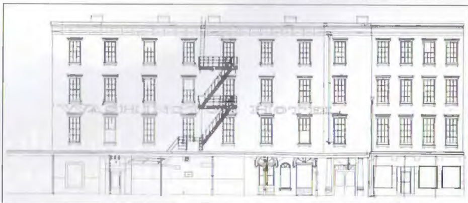
Dual cameras produce a three-dimensional image from which the computer can produce a scale drawing.
