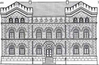
A drawing of the restored west elevation of the General Land Office was prepared by the Williams Company using a Macintoshbased CAD system.
