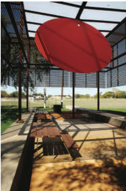
**Above and left** *The bright red mobile hangs from above and pivots according to the wind. Cast-in-place concrete piers organize the ground and serve as alternatives to wood benches and tables.*
