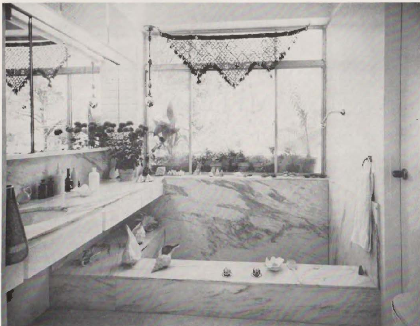
Lowering the ceiling in the kitchen below made possible a sunken tub in the beautiful, marble bath — which helped make this Swenson & Linnstaedter home a prize-winner in the "Homes for Better Living Awards" program.
